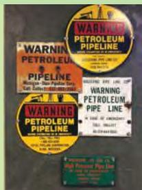
Pipeline markers are located along the pipeline route, and identify the **general** location of the line. Only a professional pipeline marker will be able to tell you the exact location of the line, and its depth. The markers also display the company operating the pipeline, type of product being transported and an emergency phone number.
